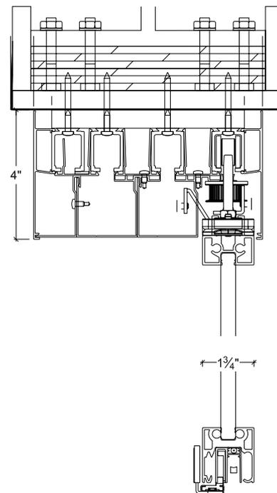
**Single glazed in the closed position with integrated handle**
