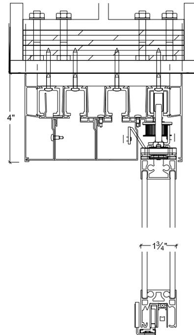
**Double glazed in the closed position with integrated handle**
