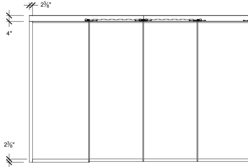
**Double glazed left stacking system with integrated handle**
