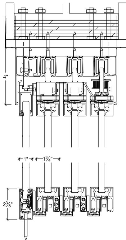
**Single glazed in the open position with integrated handle**
