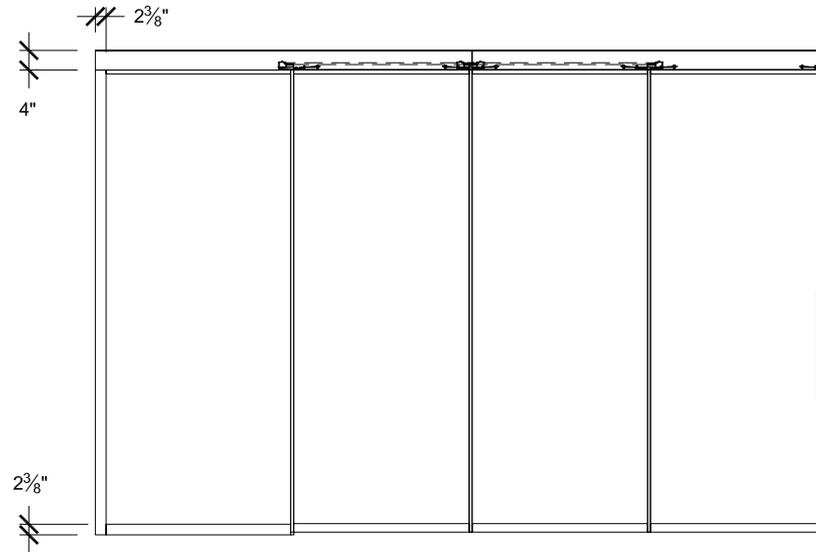
**Single glazed left stacking system with integrated handle**
