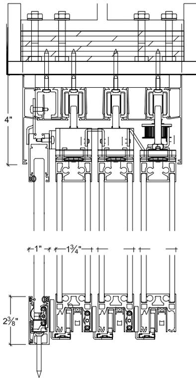
**Double glazed in the open position with integrated handle**
