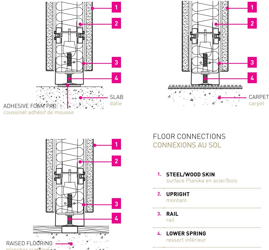
PLANIKA demising wall systems are fully adjustable adapting to any ceiling height with a total tolerance of  $+2\frac{3}{8}$ " at either the top or bottom track.
