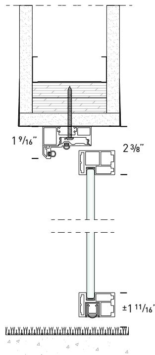
**WITH CONCEALED CLOSER & DROP SEAL IN CLOSED POSITION (OPTIONAL)**
